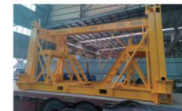
05 Self-latching overheight frame Operation: Semi-Automatic ISO container sizes: 1x20', 1x30', 1x40' and 1x45'
