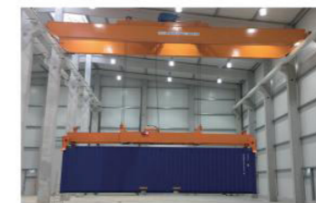
04 Electric Automatic spreader ISO container telescopic: 20'-30'-40'-45'
