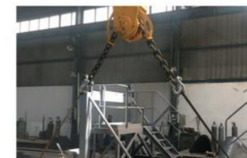
09 gravity centralizer Lifting with 40t load; Keep balance
