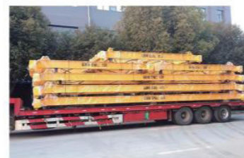
02 Frame type fixed spreader Operation: Manual, Mechanical, or Semi Automatic ISO container sizes: 1x10', 1x20', 1x30', or 1x40'
