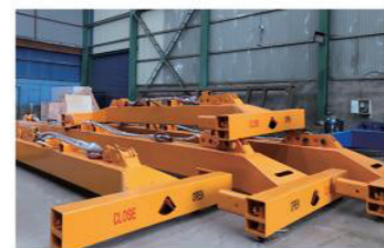
01 I type fixed spreader Operation: Manual, Mechanical, or Semi Automatic ISO container sizes: 1x10', 1x20', 1x30', or 1x40'
