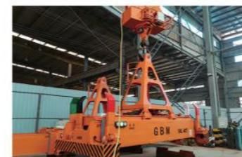
03 Hydraulic Automatic spreader Optional: Hydraulic flipper; Rotary head; Translation function ISO container telescopic: 20'-30'-40'-45'
